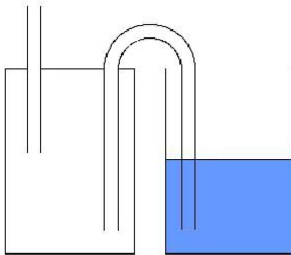
5. A U-shaped tube connects an air-filled sealed jar with an open glass of liquid. The sealed jar has a straw coming out of the top. If you sucked on the straw, what do you think would happen to the liquid?
